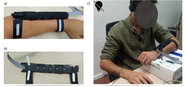
Fig. 3. Experimental setup: a) observer's view of the device fastened to the dorsal part of the forearm, b) the bottom part of the device in contact with the skin, c) an observer simulating the experimental setup in normal light conditions.
